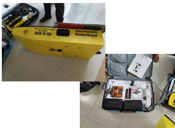
Photo 2.2.4 Radio Control Boat for Surveying the Riverbed
