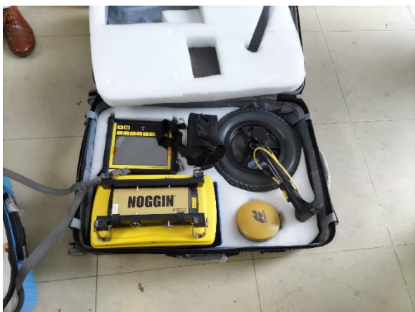
Photo 2.2.1 Portable Ground Penetrating Radar
