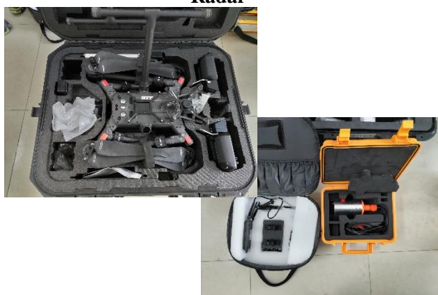
Photo 2.2.3 Drone and Survey Equipment with LiDAR and Single beam
